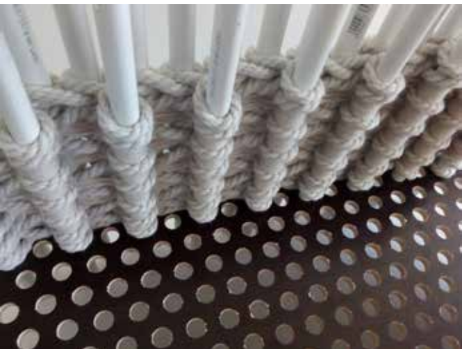
Multiweave structure with and without the warp supports.
