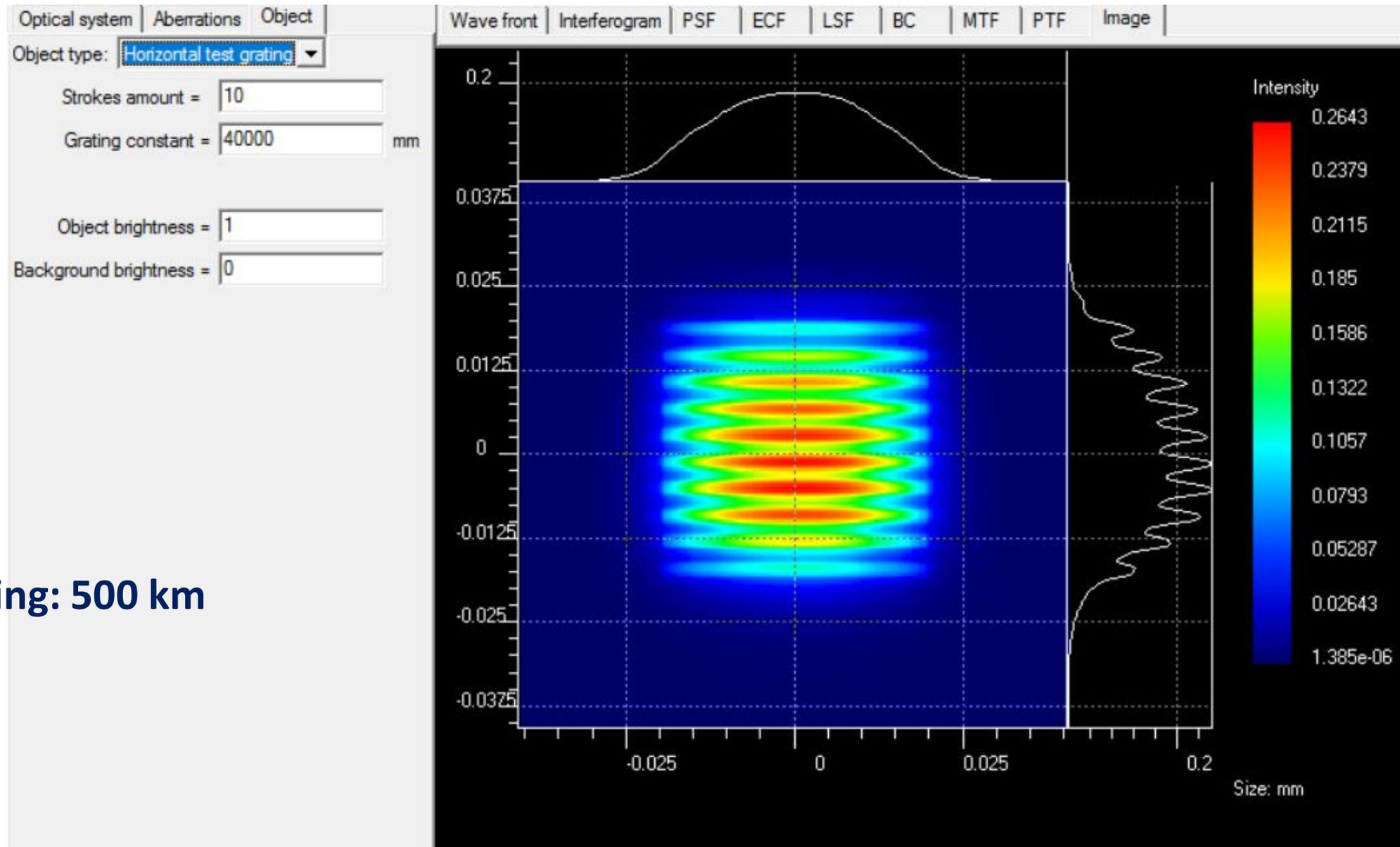
Figure 5. X test grating image
