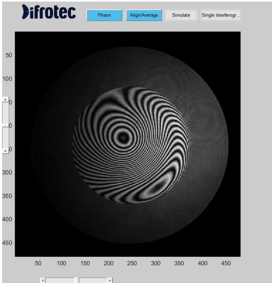
*Figure 7. Interferogram of the on-axis beam*
