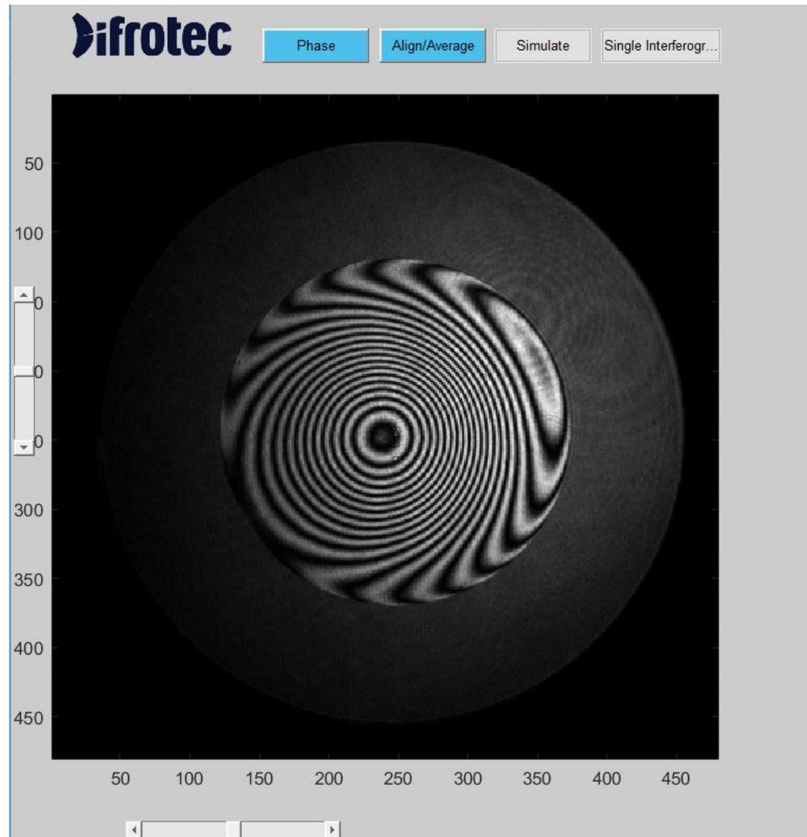
*Figure 1. Interferogram of the on-axis beam*
