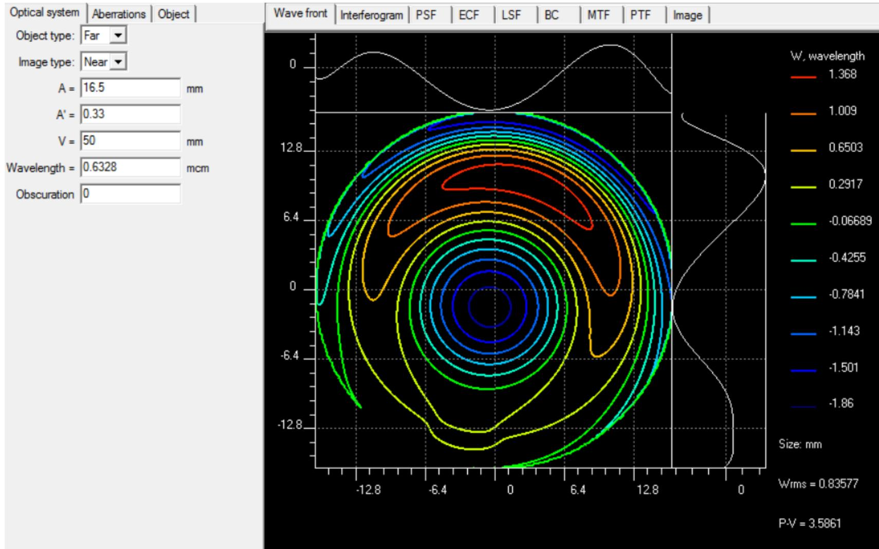
Figure 8. Wavefront diagram
