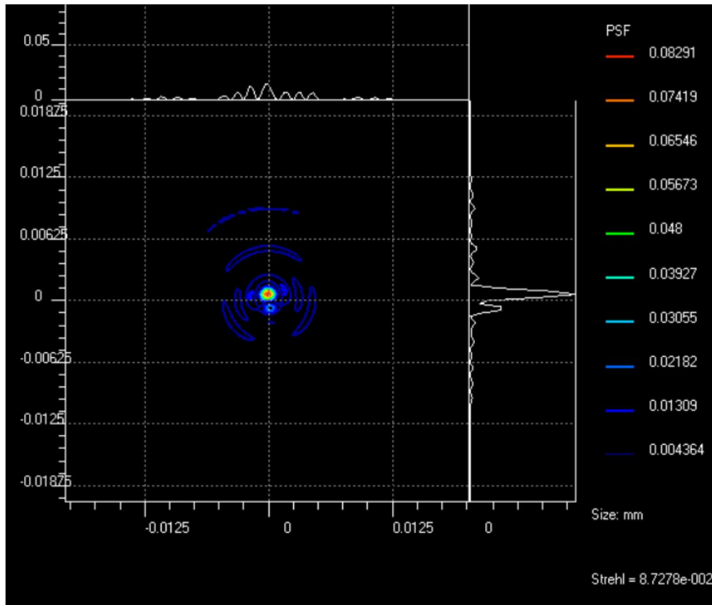
Figure 3. Point spread function
