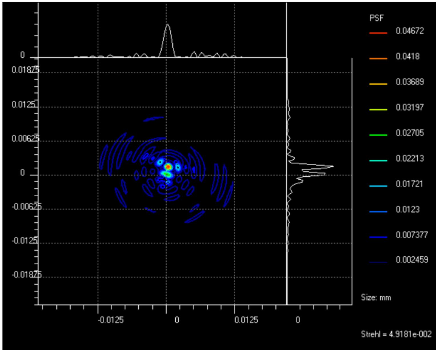
Figure 9. Point spread function
