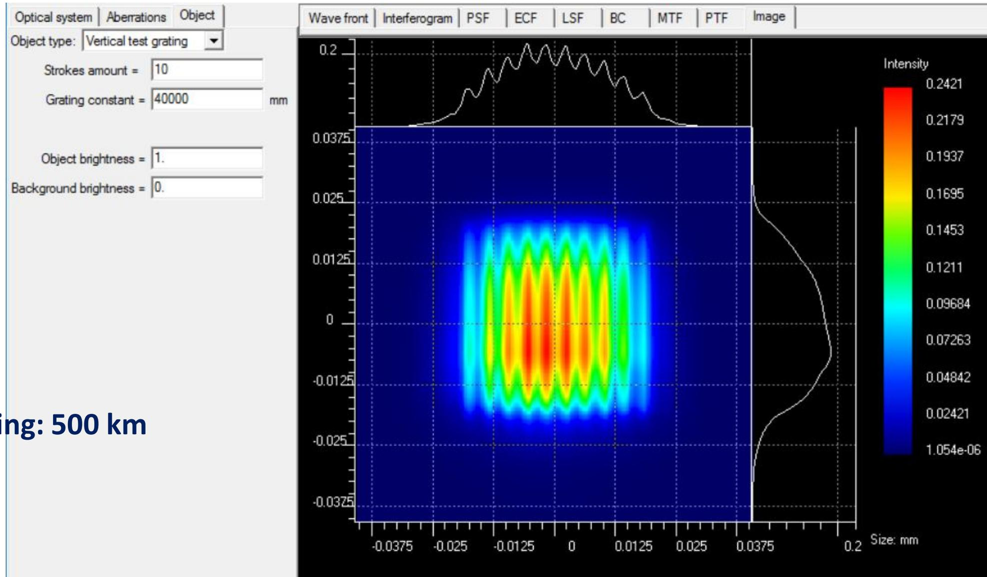
Figure 10. Y test grating image
