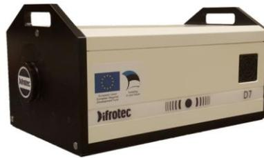
The D7 can help you easily detect the absolute figure of a surface or wavefront which in other kinds of interferometers is masked by the errors of a physical reference. **Absolute figure means that the measured form is counted from the absolute reference i.e. perfect spherical wavefront produced by diffraction of light by a sub-wavelength aperture.**
