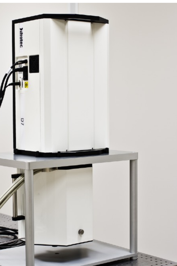
D7 & sample stage arranged in vertical position
