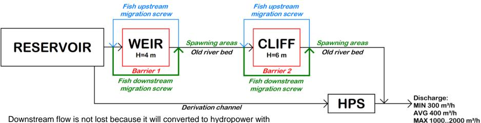
VSD controlled generator. Installed power (kW):  $P = Q \times H \times 7,2$
