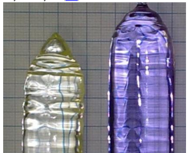
Figure 2. Ba and Sr Tungstate-Molybdate crystals for Raman shifting.
