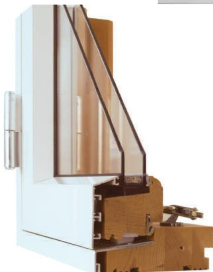
A three-layered window are protected with aluminium profiles. To reduce heat loss at the edge of the glass, we recommend using an insulated glazed unit that has SWS (plastic) spacers rather than the traditional metal.
