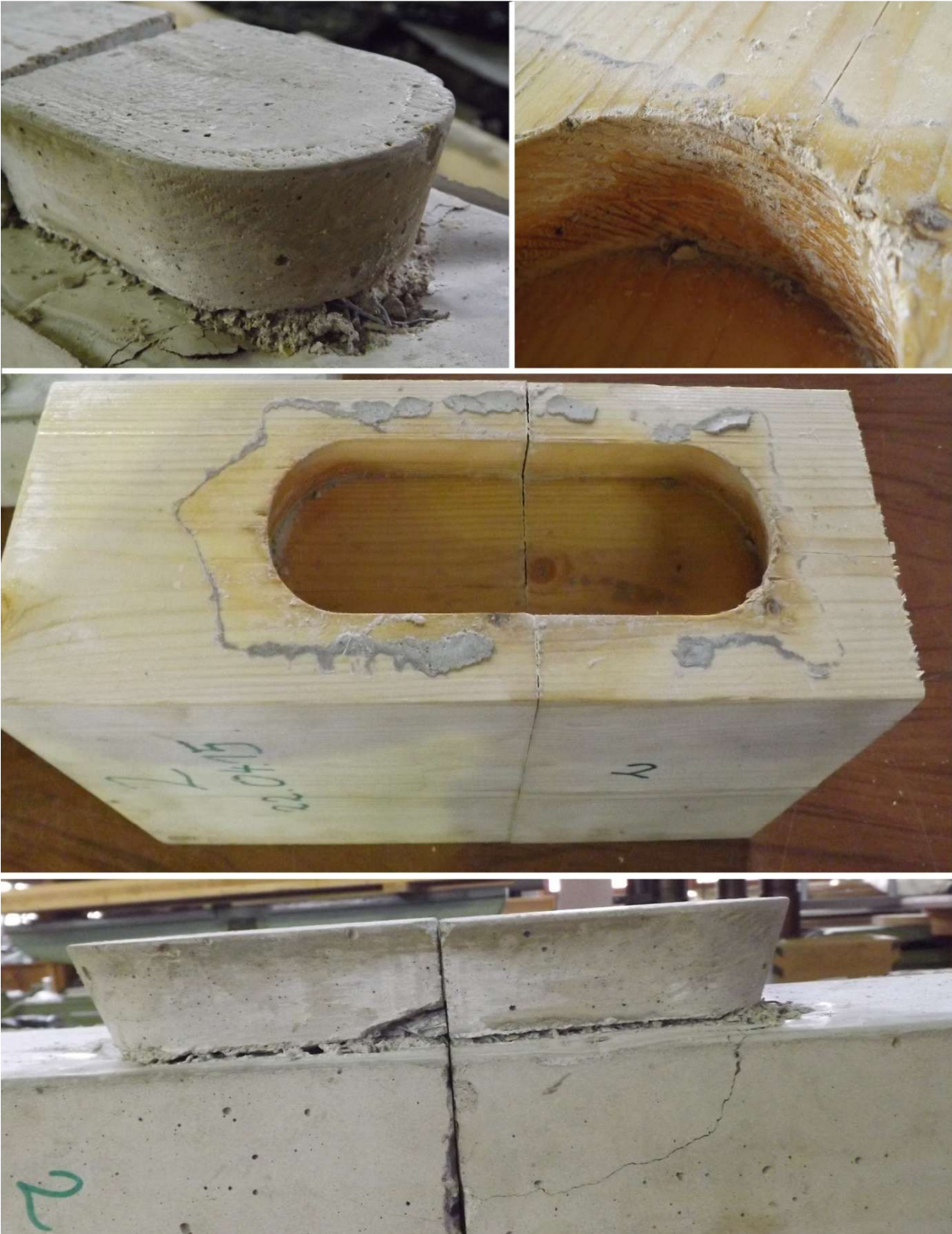
Katsekeha 2 - betoontapi rabe purunemine
