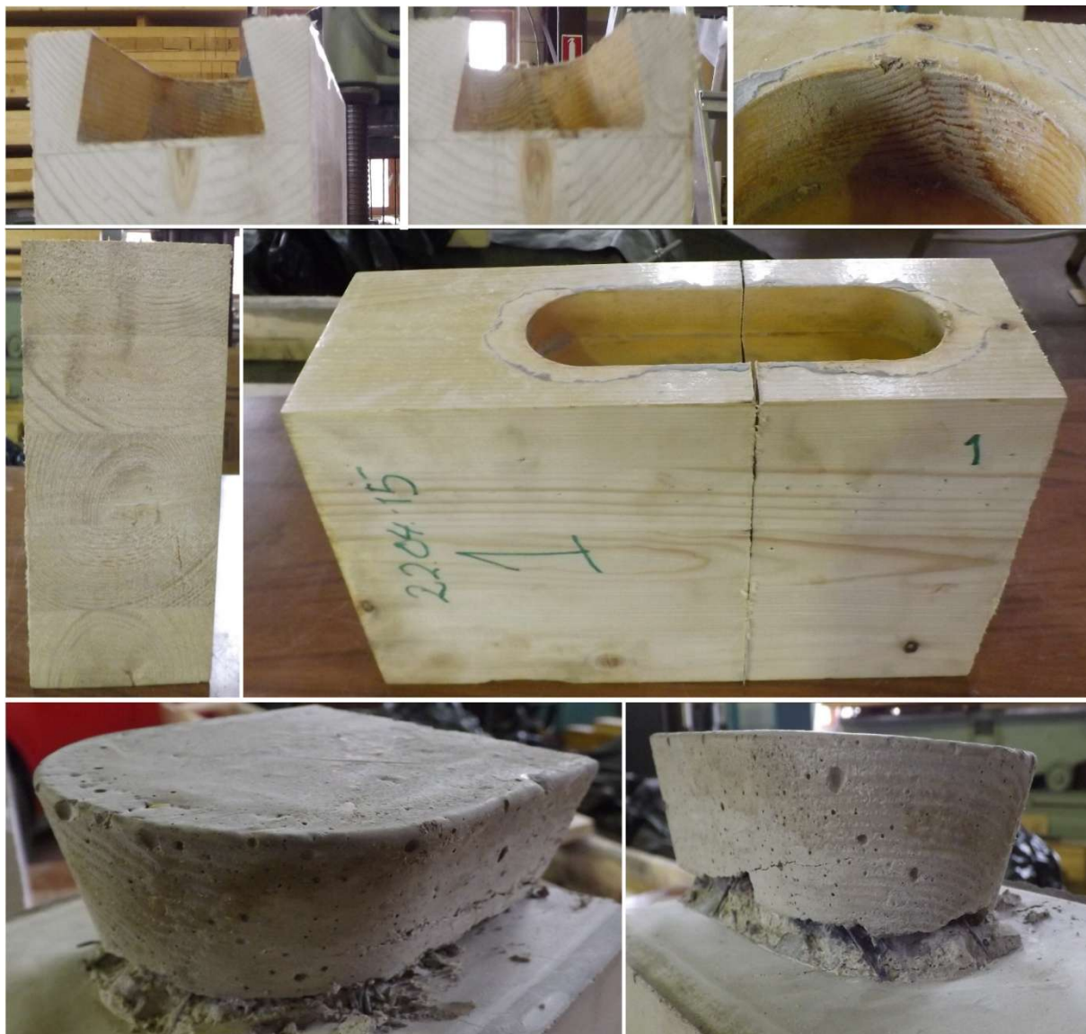
Katsekeha 1 - betoontapi rabe purunemine
