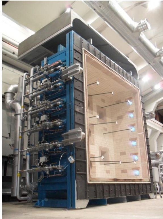
Figure 9 - Full-scale fire testing furnace [36]
