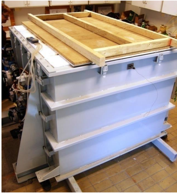
Figure 8 - Model scale furnace at SP Technical Research Institute of Sweden [7]
