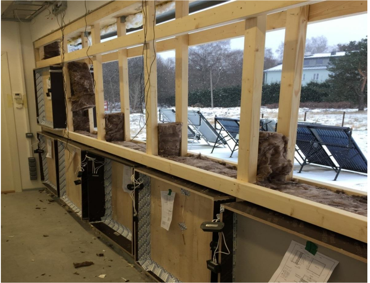
Figure 2.8: Picture showing test walls already mounted in technological test facility
