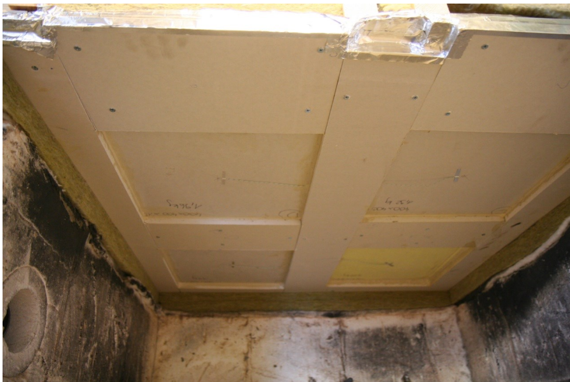
Figure 4.10 – Test specimen T 3 mounted on the furnace (view of exposed side)
