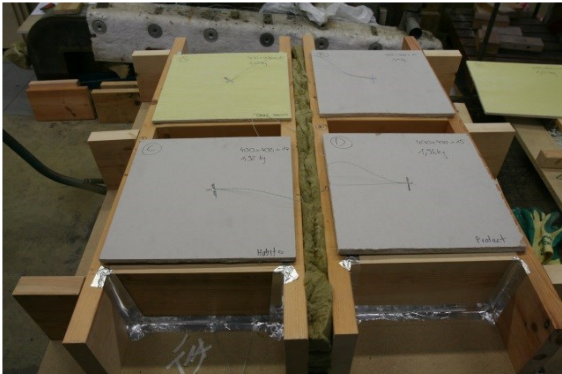
Figure 4.5 – View of specimen T_3 during assembly (gypsum boards attached)
