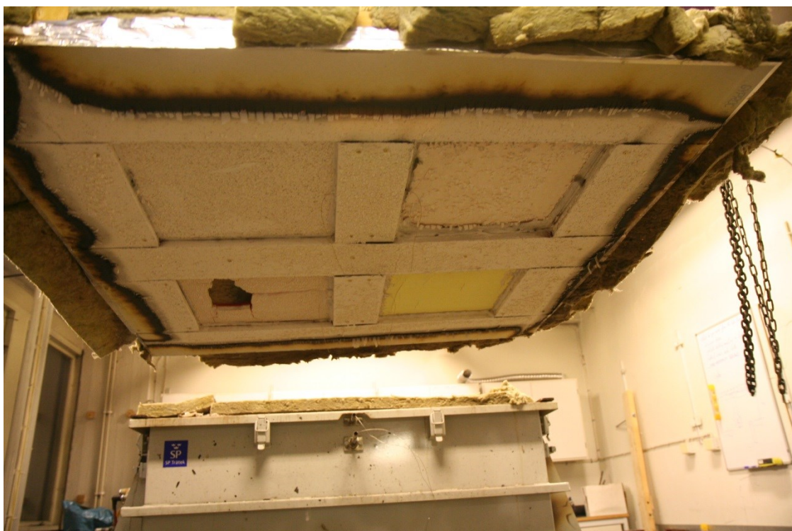
Figure 4.11 – Test specimen T 2 after removal from furnace
