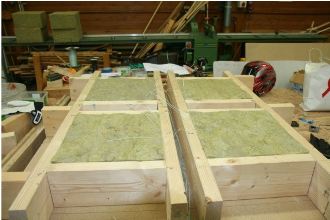
Figure 4.4 – View of specimen T_3 during assembly
