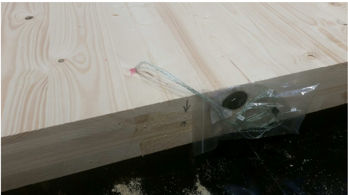
Figure 3.5. Finished CLT panel
