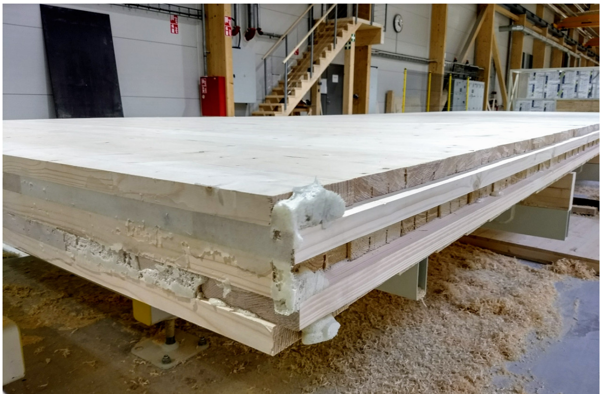
Figure 3.3. CLT panel prior to machining
