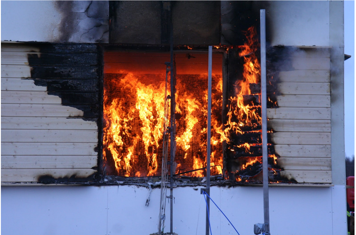
Figure 2.18 The second layer of CLT is burning
