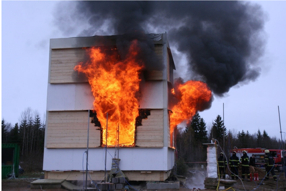
Figure 2.15 Fire has spread to the facades
