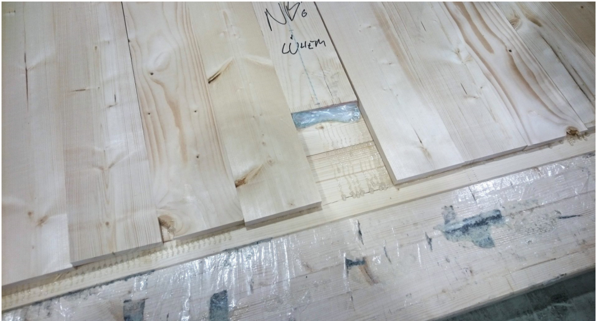
Figure 3.4. Thermocouples were put away before CNC machining
