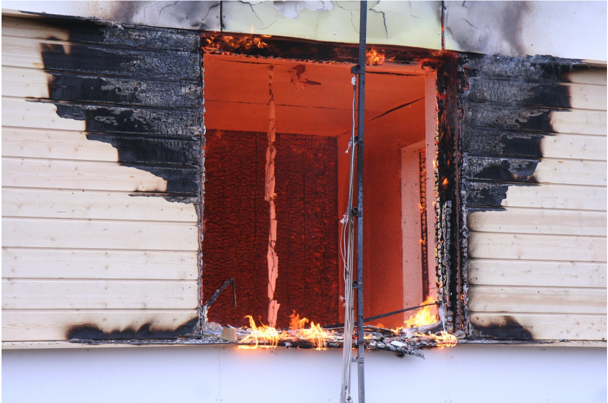
Figure 2.17 The CLT is smouldering
