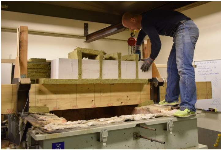
Figure 20. Fixing light concrete blocks on top of the beam.
