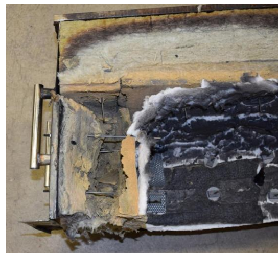
Figure 28. Result of exposing wool sheets to fire alongside.
