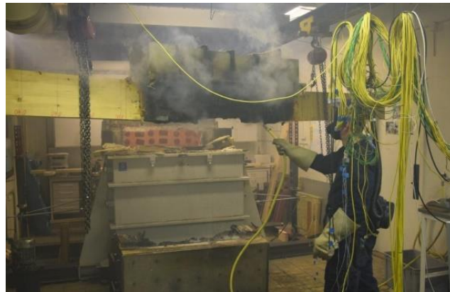
Figure 39. Extinguishing the specimen
