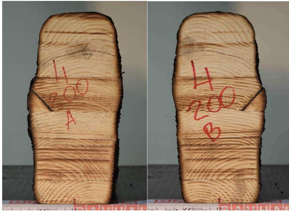
Figure 42. Mirrored shapes of the faces of the same cut. Presented using specimen 4, cut at 200cm from reference starting point “0”.
