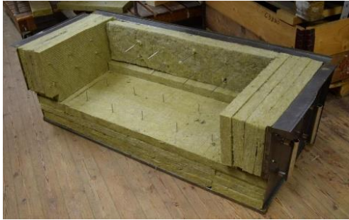
Figure 26. Placing stone wool insulation on a furnace cover.
