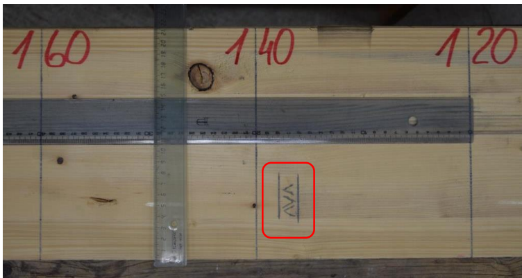
Figure 101. Failure zone of Beam 6 face "C" before the fire test. Finger joint location at 1360mm is marked with red.
