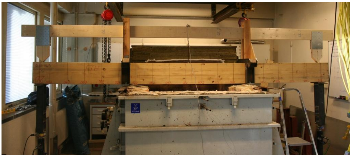
Figure 30. Test set-up: specimen positioning, supports, load application, displacement.
