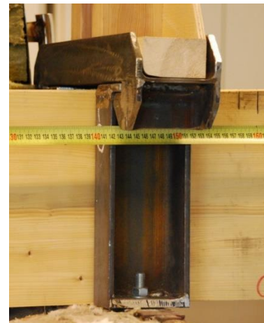
Figure 17. Support details on furnace's
