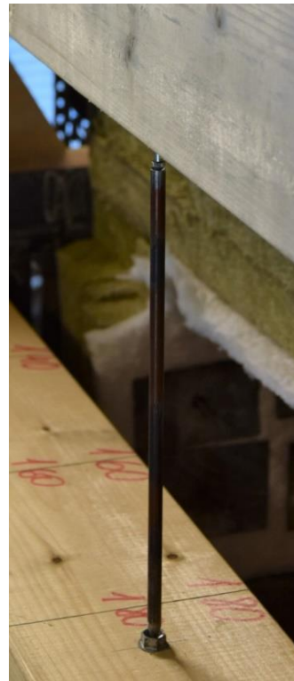
Figure 25. Steel rod between LVDT and lag screw.
