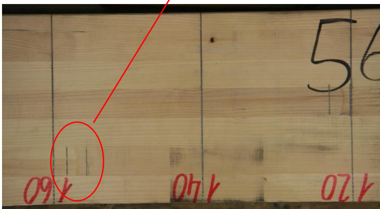
Figure 80. Failure zone of Beam 3 face "B" before the fire test.
