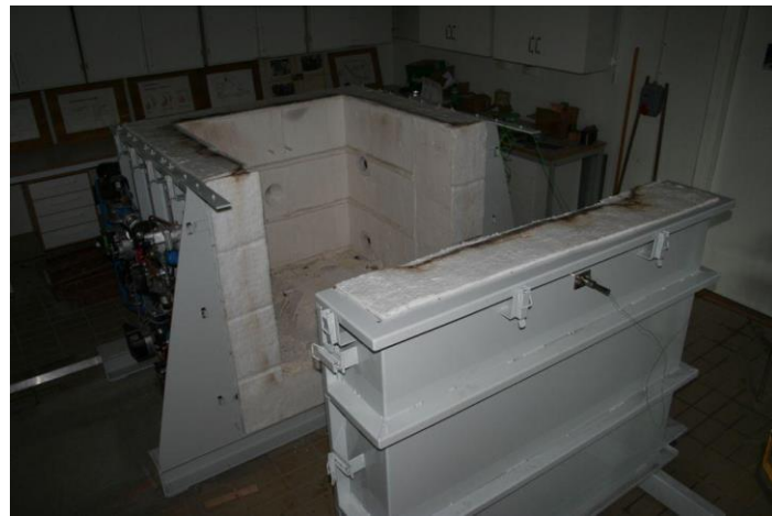
Figure 14. Furnace's removable front and inner ceramic fibre insulation. Photo: SP
